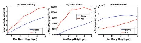
Fig. 8 Effects of the protrusion height on swimming for van Haastert's and Barry's cell:  $\mathbf{a}$  mean velocity  $\sim$  maximum protrusion height;  $\mathbf{b}$  mean power  $\sim$  maximum protrusion height;  $\mathbf{c}$  performance  $\sim$  maximum protrusion height
