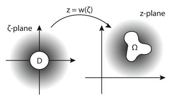
**Fig. 1** The conformal mapping from  $\overline{\mathbb{C}}/D$  to  $\overline{\mathbb{C}}/\Omega$
