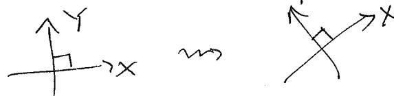
via  $\begin{bmatrix} X' \\ Y' \end{bmatrix} = Q \begin{bmatrix} X \\ Y \end{bmatrix}$  for some orthonormal  $Q$ , i.e.  $Q^T = Q^{-1}$
