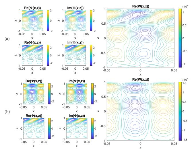
FIG. 8. Streamlines and the vorticity field for the perturbation modes with the largest eigenvalue. (a)  $\mathcal{E}_r = 1000$ ,  $\mathcal{R}_e = 5$ ,  $\ell = 0.2$ ,  $\omega = 75$ , and  $\mathcal{A} = -200$ . (b)  $\mathcal{E}_r = 1000$ ,  $\mathcal{R}_e = 5$ ,  $\ell = 0.2$ ,  $\omega = 75$ , and  $\mathcal{A} = -10$ .
