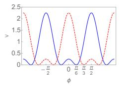
FIG. 4. Potential energy corresponding to Eq. (54), with  $|\frac{\gamma_1}{\gamma_2}| = \frac{1}{2}$ , for extensile (dashed line) and contractile fibers, respectively. The unstable rest states for each type of fiber correspond to  $\phi = \frac{\pi}{2}, -\frac{\pi}{2}$ . The stable stationary flows, with uniform director, correspond to  $\phi = \frac{\pi}{3}, \frac{\pi}{6}$ , for the extensile and compressible systems, respectively.
