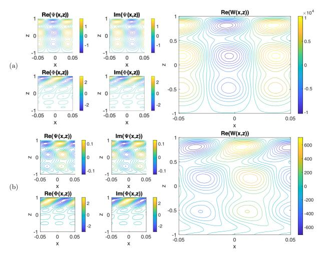
FIG. 9. Streamlines and the vorticity field for the perturbation modes with the largest eigenvalue. (a)  $\omega = 75$ ,  $\mathcal{R}_e = 0.1$ ,  $\ell = 0.2$ ,  $\mathcal{E}_r = 1000$ , and  $\mathcal{A} = -200$  and (b)  $\omega = 75$ ,  $\mathcal{R}_e = 5$ ,  $\ell = 0.2$ ,  $\mathcal{E}_r = 100$ , and  $\mathcal{A} = -200$ .
