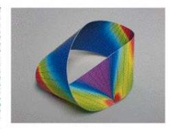
Figure 1 Photo of a paper Möbius strip of aspect ratio 2n. The strip adopts a characteristic shape. Inextensibility of the material causes the surface to be developable. Its straight generators are drawn and the colouring varies according to the bending energy density.
